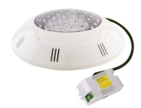
Wall mounted niche less lights are built of stable, heat-resistant plastic materials. This flood lamp has been designed to be used fully submerged it is a class III electric part with low safety voltage & complies with IPX8 degree protection at a normal depth of 2meters. Cross head mount with screws are supplied as part of light to fix in the wall. This light comes with high quality LED bulb, GEL filled for long life of product.
